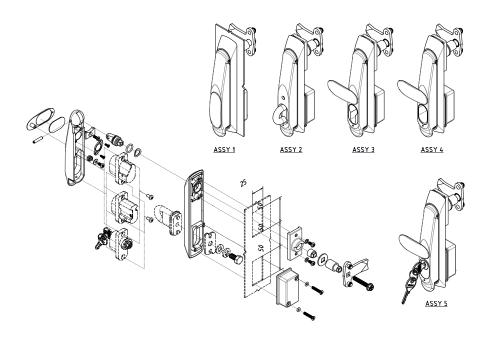
Selectlok's new SwitchUp system makes choosing, fitting and replacing swing handles even easier. Our new high quality swing handles are modular, allowing your most popular lock inserts to be easily changed without having to replace the handle.
