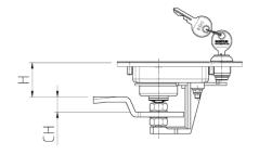
Cam assembled in Stainless steel dish folding T handle
