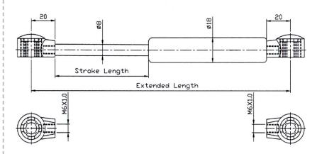
Stainless steel ball ends supplied separately. (Part no: SW-13-SS)
